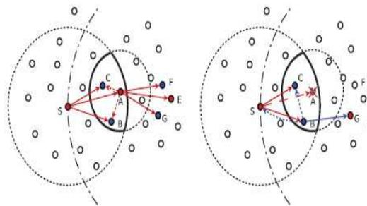
Figure1: Operations of POR in Normal Situation
