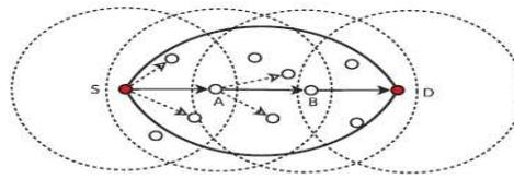
Fig 2: Duplicate Relaying Is Limited In The Region Enclosed By The Bold Curve
