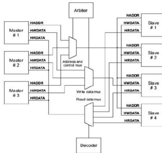
Figure 5. AMBA AHB Arbitration Block diagram
