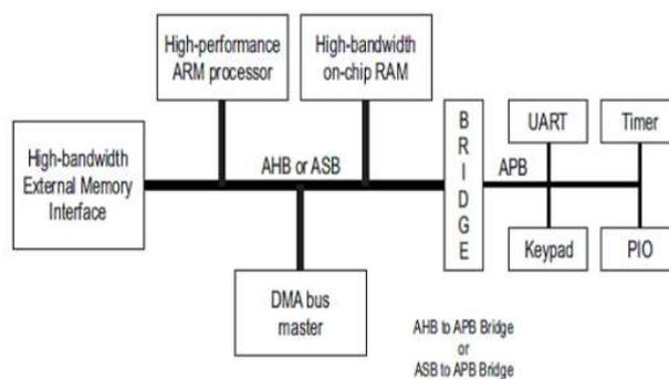
Figure 4. AMBA based Simple Microcontroller.
