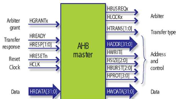
Figure 2.AHB master signal splitter
