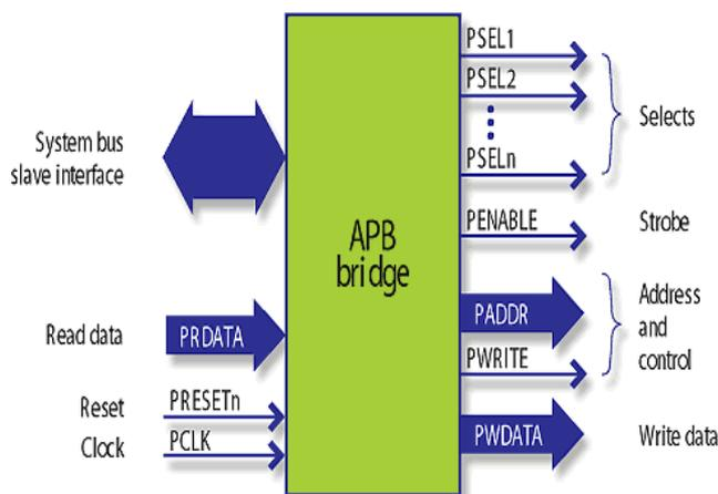
Figure 3. Advanced Peripheral Bus Bridge
